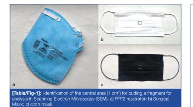
of each specimen at magnifications of 100, 500 and 1000x. The distance among threads was determined by EDS.
