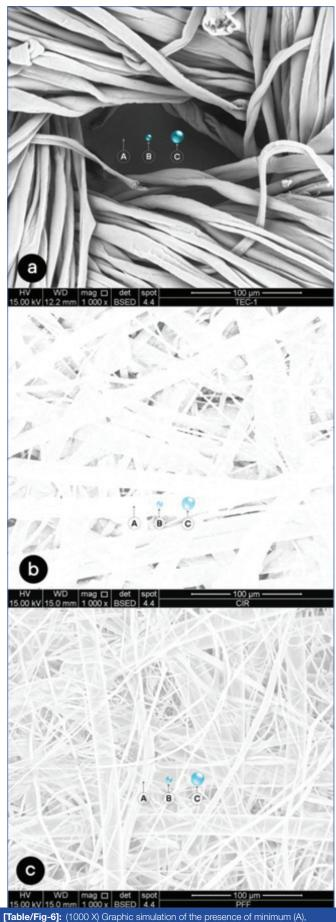
**[Table/Fig-6]:** (1000 X) Graphic simulation of the presence of minimum (A), intermediate (B) and maximum (C) size droplets in relation to the space of specimen fibrils of cloth mask (a), surgical mask (b) and FFP2 respirator (c)
