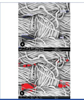
[Table/Fig-2]: (500 X) Photomicrographs of cloth mask. a) visualisation of distance among threads; b) gap spaces (red mark).
